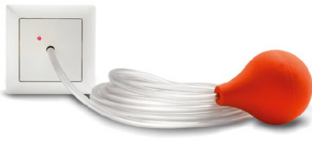
Pneumatic call unit with pneumatic switch element. Call release through squeezing the red rubber ball on 2 m long clear plastic tube
